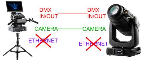
Simplest Setup, Robospot Station controls Fixture with no input from the console. Address the fixture to channel 1 (or any other valid address). Once the Fixture and the Station are connected, the RDM discovery feaure of the station will find the fixture.
